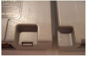
In order to get them in, a modification has to be made to the case by removing the tabs in the cartridge slot:
