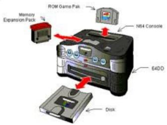
This terrible Nintendo commercial failure was intended to overcome the initial size limitations of cartridges (more expensive though faster than discs) and included a proprietary floppy disk-like magnetic media:
