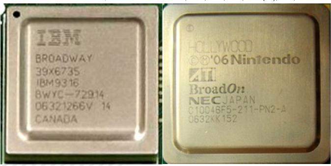
On the one hand the IBM Broadway CPU at its side the ATI Hollywood GPU.
