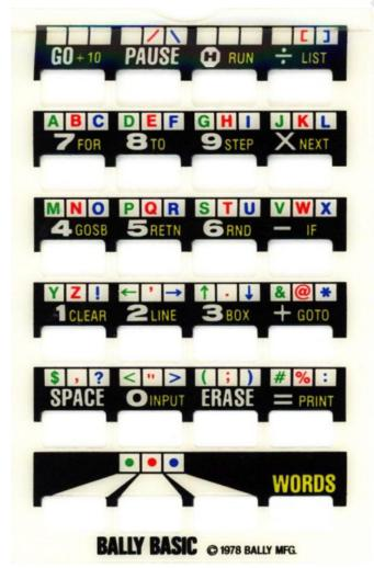
Fig. 9 - The template to be attached to the console keypad in order to enter programs in BASIC (source: thedoteaters.com)
