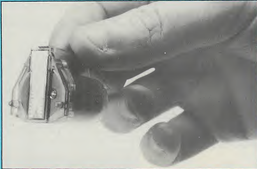
The print head from HP's ink-jet printer contains 3ml. of ink, which is ejected under pressure through a row of 12 tiny nozzles.
