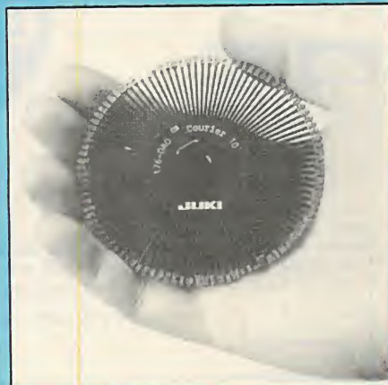
A typical daisywheel has 96 characters mounted on the end of flexible stems.
