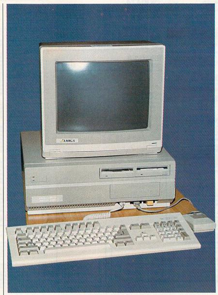
Commodore's new Amiga 2000 computer is an expandable powerhouse machine that features both Amiga and IBM card slots; up to nine megabytes of RAM; a flexible combination of 31/2-inch, 51/4-inch, and hard disk slots; a reconfigured keyboard; and the ability to run IBM and Amiga software simultaneously.
