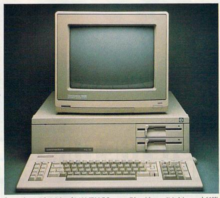
Commodore's PC10-2 is a \$1,199 IBM PC compatible with two disk drives and 640K of RAM. The PC10-1 (not shown) is priced at \$999 and contains one disk drive and 512K of RAM (expandable to 640K).
