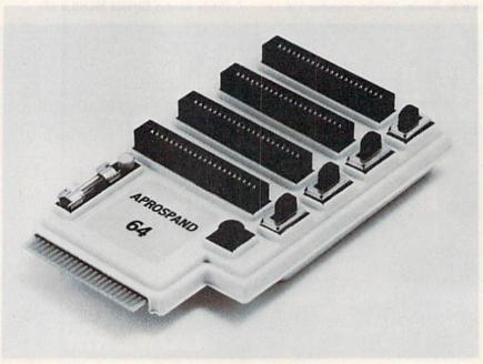
jacks, computer connecting cable, and | Aprospand 64 is a four-slot cartridge expander for the Commodore 64.
