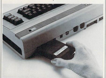
The Final Cartridge, from H & P Computers Of America, is an external operating System for the Commodore 64.
