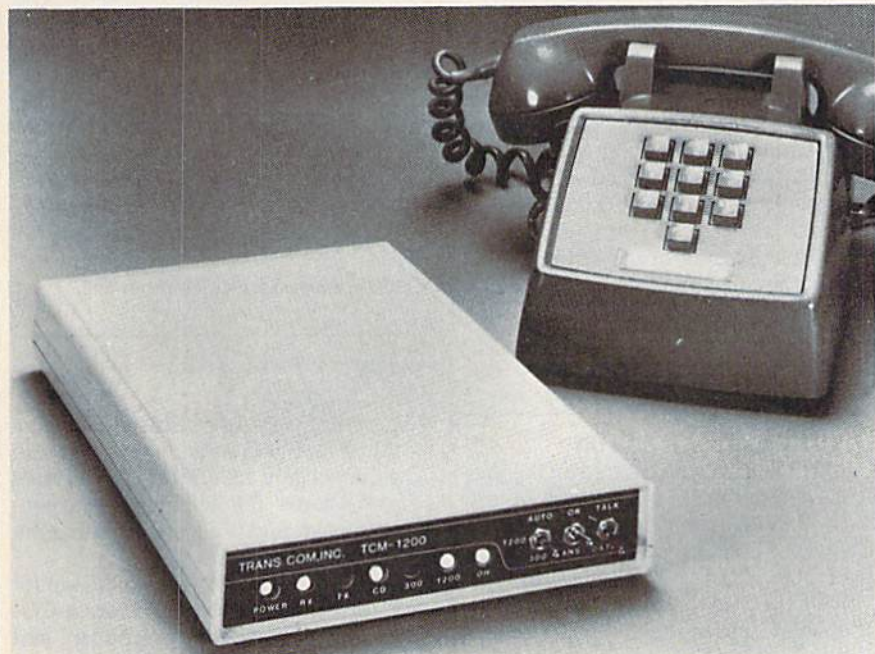
The TCM-1200 is a 300/1200-baud direct-connect modem for the 64 and 128.
