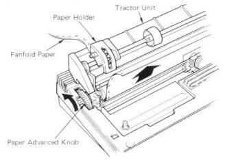
b) Adjust the sprocket position to fit with paper width. If the sprocket pins do not engage with the sprocket holes, move the paper holder to fit. Close the paper holder cover and push the paper release lever to OPEN.
