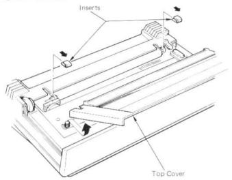
b) Insert the front hooks of the tractor unit into the holes where the inserts were located previously, and securely fix the unit onto the platen shaft. Engage the rear hooks to the holes at the back of the printer.
