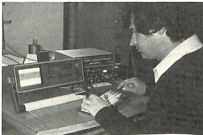
W.A. radio salesman Tom Barrett using a Commodore SX-64 portable computer to send and receive error-free written messages to a mining camp via 2-way radio.
